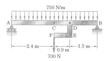
A beam AB under loading is shown in the figure. The rigid bar DEF is welded at a point D. The Young's modulus of the beam material is 200 GPa and its moment of inertia is  $20 \times 10^6 \text{ mm}^4$ .
