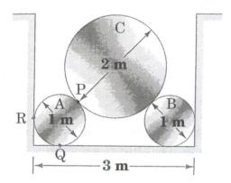
A cylinder C weighing 1000 N is supported by two cylinders A and B weighing 500 N each as shown in the figure. Calculate the contact forces at P, Q and R.
