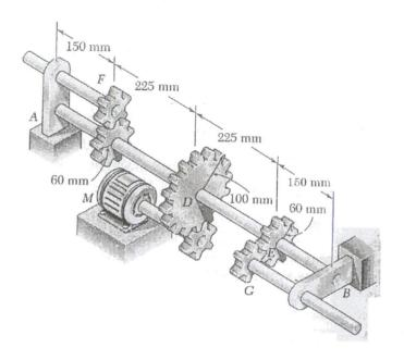
A solid shaft AB rotates at 450 rpm and transmits 20 kW from the motor M to machine tools connected to gears F and G. A power of 8 kW is taken off at gear F and 12 kW is taken off at gear G. The allowable shear stress is 55 MPa. Determine the smallest permissible diameter of the shaft AB.
