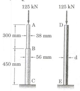
The aluminium rod ABC having Young's modulus 70 GPa consisting of two cylindrical portions AB and BC, is to be replaced with a cylindrical steel rod DE with Young's modulus 200 GPa of same overall length. Determine minimum required diameter, d, of the steel rod if its vertical deformation is not to exceed the deformation of aluminium rod under the same load and if the allowable stress in the steel rod is not to exceed 165 MPa.
