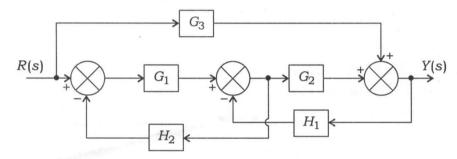
Evaluate the overall transfer function  $\frac{Y(s)}{R(s)}$  using block diagram reduction technique.
